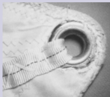
Webbing hand sewn with doubled waxed thread with a no. 13 needle. Be sure to 'pre-tension' the webbing when it is stuck down with double sided tape, to ensure the load is being taken by the webbing.
