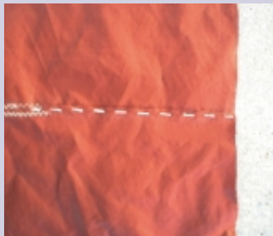
Frayed edge heat sealed, the two sides double-sided taped and tack stitched together.
