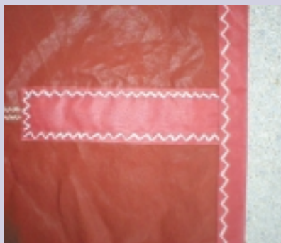
Reinforcing patch taped and hand stitched. Leach tape re-established. For this job use a small (approx no. 16 needle) and single waxed thread.
