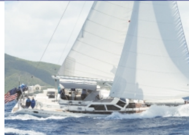
Photo 1 Example of slack main halyard and very slack genoa halyard
